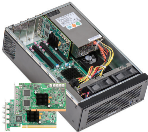
HDMI add-in card DisplayPort 1.1 add-in card
