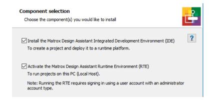
IMPORTANT when installing on a Matrox 4Sight GPm: After installing Design Assistant, the next reboot may start a firmware (FPGA) upgrade. If you get a message telling you that DesignAssistantRuntimeMonitor is using MIL, then you must use the Task Manager to kill the DesignAssistantRuntimeMonitor process so that the upgrade can continue.
