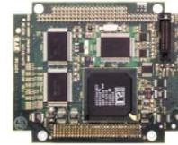
Matrox Meteor-II for PC/104-Plus™ (PCI frame grabber)
