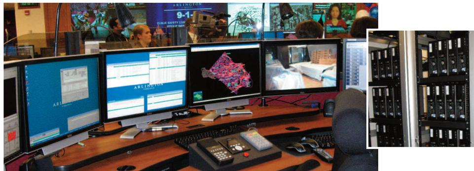
*Matrox Extio PCI transmitter cards installed in systems in temperature-controlled room down hall from ECC. The RGU can be located up to 820ft (250m) away from the host PC.*
