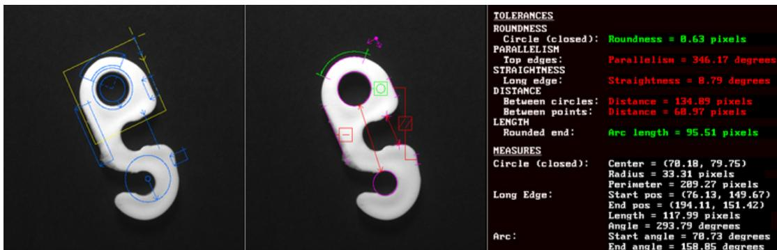
The Matrox Imaging Library Metrology module analyzes the image of a machined hook. Based on its features, the metrology results determine that the part falls outside the accepted tolerances. Image courtesy of Matrox Imaging
