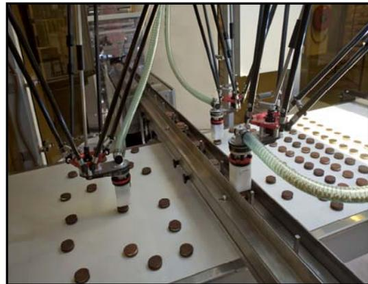
Vision-guided robots is quite common. The camera acquires an image, and software processes the image. In this cookie sorting application, the robots place different shaped cookies into a blister tray for packaging. The imaging software will help determine the correct shape of the cookie, index it so as not to overfill the tray, and send coordinate information to the robot. Images courtesy of Bosch Packaging Technology.
