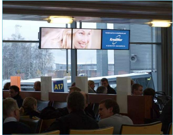
Clear Channel set up 42 computers throughout Oslo airport, each connected to a TripleHead2Go unit outputting to three 40" NEC LCD monitors with slim bezels. On some of the triple-screen setups, advertising content was designed to stretch across the three screens. On others, each monitor displayed independent content, such as local, international, and translated newscasts.
