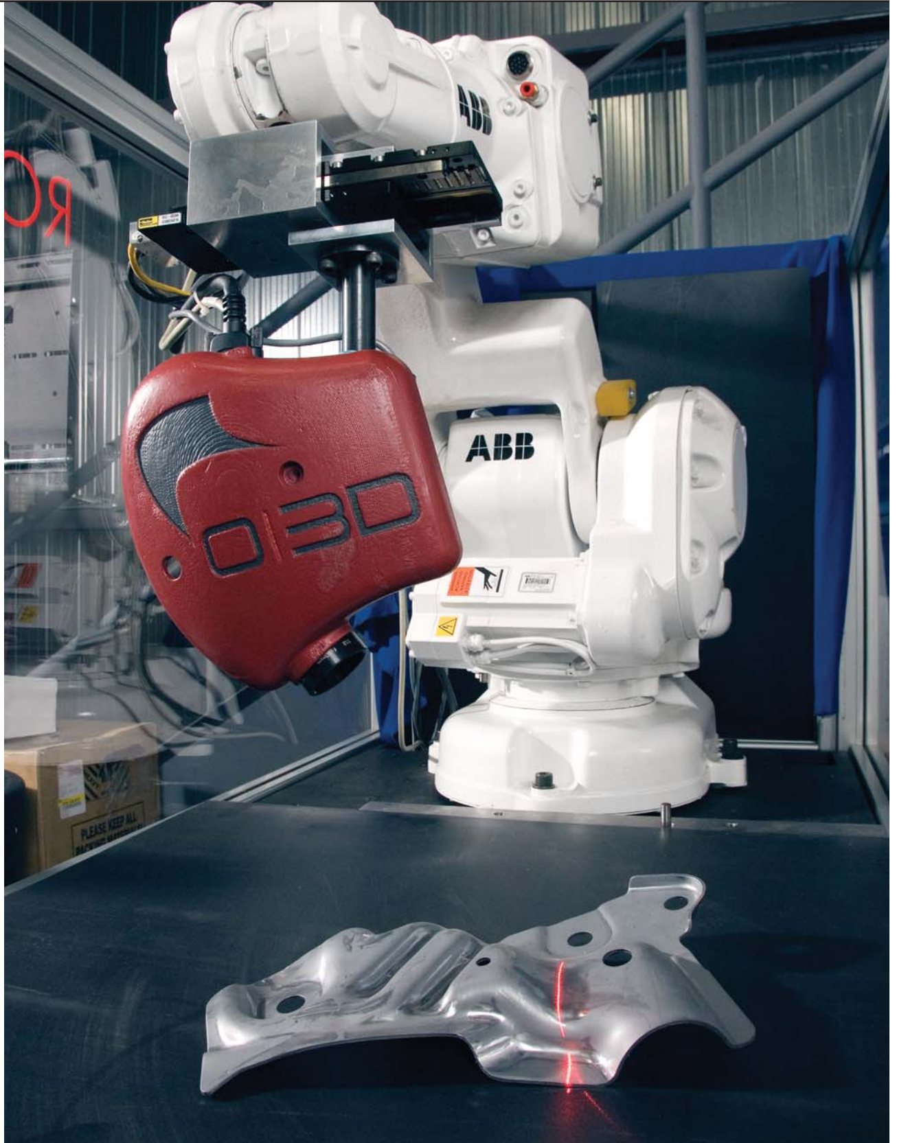
This ABB IRB-140 robot acts as a positioning device that allows 3D scanning.
