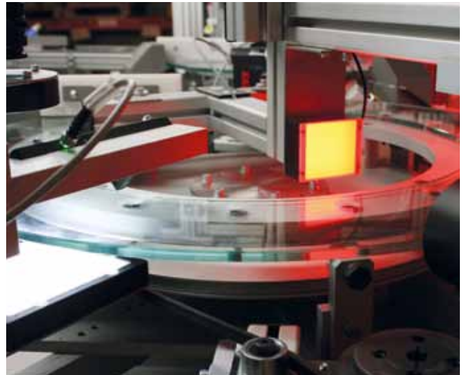
Plastic component camera inspection system
